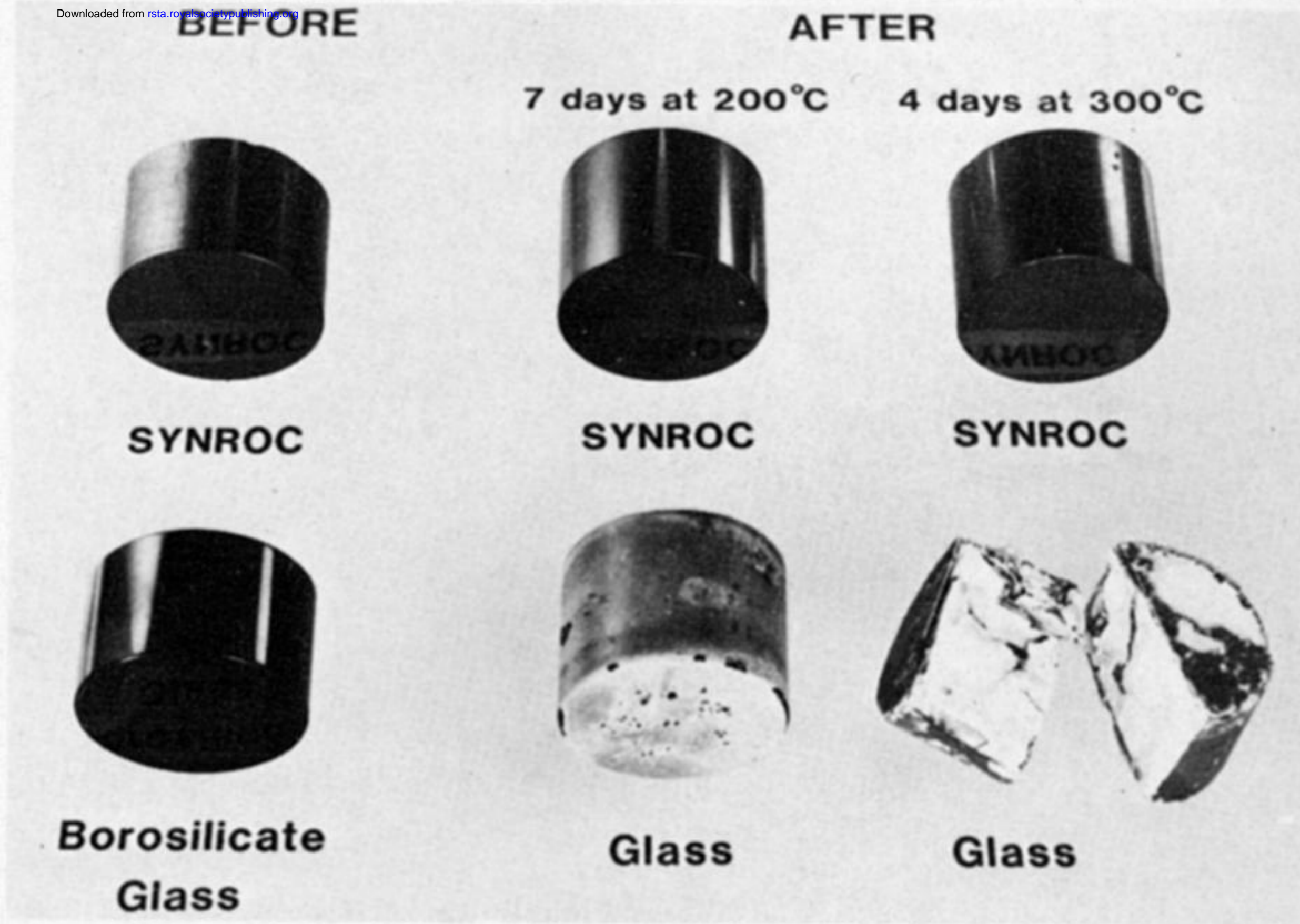
FIGURE 5. Comparative leaching behaviour of 5 cm diameter cylinders of SYNROC and borosilicate glass, both containing simulated HLW, in water at 200 and 300 °C.
